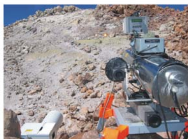
UV-DOAS and TDL systems for SO 2 and CO 2 measurements in the air atmosphere inside the summit crater of Teide volcano
