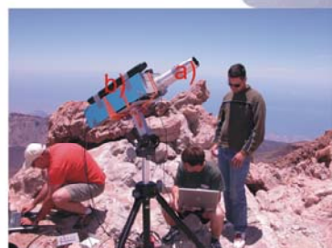
SO 2 flux measurements by means of COSPEC and miniDOAS in stationary mode at the summit crater of Teide volcano.
